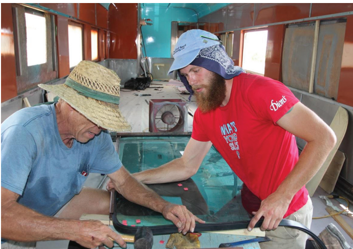
Glass expert Steve Laube, left, assisted by son Steve Jr., installs a rubber gasket around one of the Cedar Park 's 26 new windows. The car's Santa-Fe-themed paint scheme is evident.
