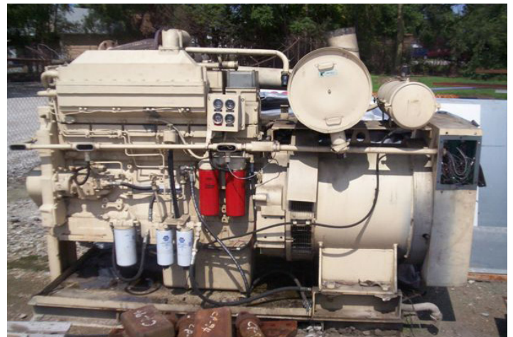
The 800-kilowatt Cummins generator being considered by ASTA for providing reliable head-end power to the trains. The unit last served in a commuter locomotive in Maryland, and would be mounted in a former MP express car.
