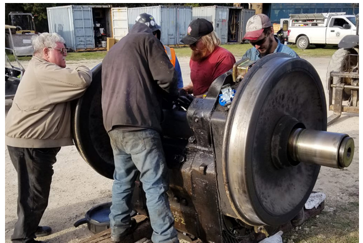
Chris Hoff leads volunteers working on a crucial job, replacement of a new traction motor powering ASTA's leased locomotive HZRX 3134.
