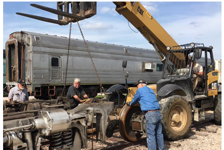
Volunteers Brian Urban, Rich Wise and Dave Shannon help the general superintendent in positioning a wheelset under the trucks of the Rippling Stream lounge-sleeper.
