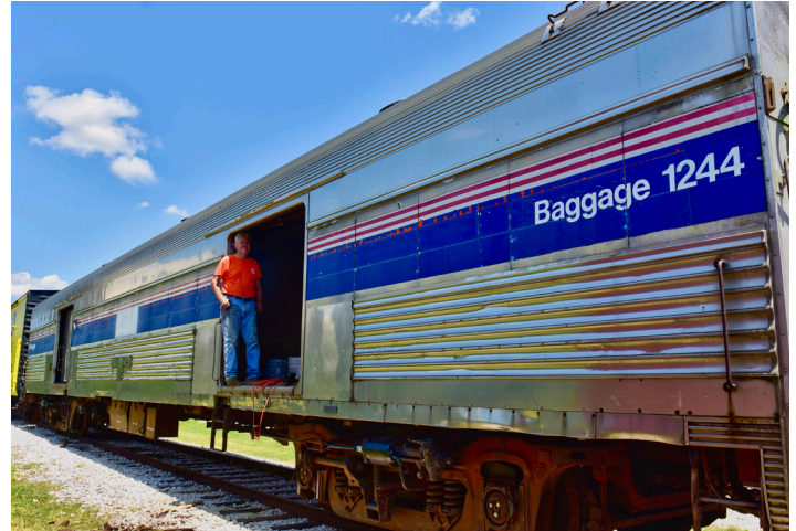
ASTA mechanical volunteer Bennie Kirk in a doorway of newly acquired baggage car 1244, being overhauled to carry the new 450-kilowatt generator for train power. (Marc Opperman photo)
